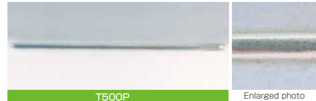
SUS304 stainless steel plate of 0.3 mm in thickness by butt joint. Welding conditions: Base current set to 2A, Pulse current set to 10A, and Pulse frequency set to 999 Hz
